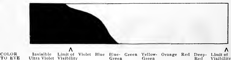
FIG. 23. ABSORPTION OF CORRECT FILTER
